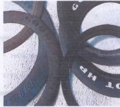
Sidewalls With & Without Beads
